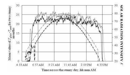
Fig. 2 Mean values of  $\Delta T = T_{glass} - T_{amb}$  for June (— black solid) and July (— grey solid) versus normalised time during few sunny days against a background of the mean values of solar radiation intensity for June (… black dashed) and July (… grey dashed)
