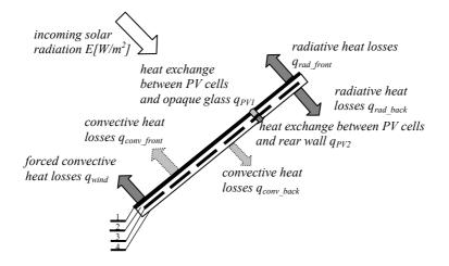
Fig. 1. Heat transfer between PV module and environment: *1* - low iron glass, *2* - EVA, *3* - PV cells, *4* - back surface (Tedlar®, glass, polyester)
